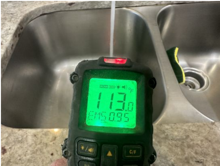
Water heater temperature.
